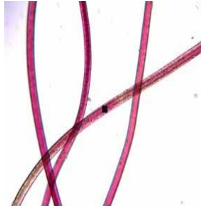
Figure 20 An example of the use of microspectrophotometry on fiber UV/VIS analysis
