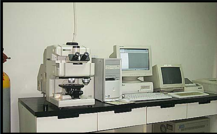
Figure 24 Microscope coupled with a Fourier Transform Infrared Spectrometer
