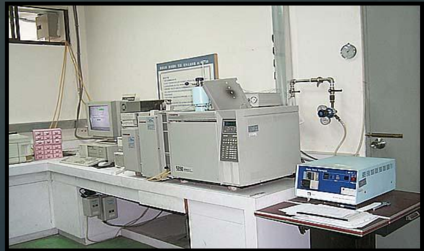
Figure 25 A pyrolysis – gas chromatograph/mass spectrometry
